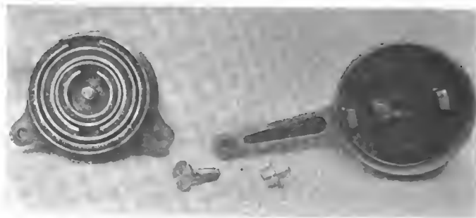
Sphinx Shock Absorber Dismounted to Show Parts
